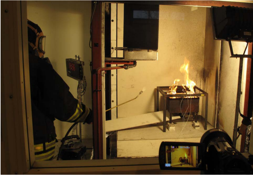
Figure 7 Applying water test 3
